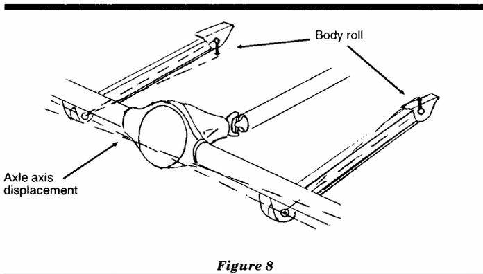
If the frame moves down one inch on one side and up one inch on the other due to a pavement undulation (or gust of wind, etc.), we have the following happen:
