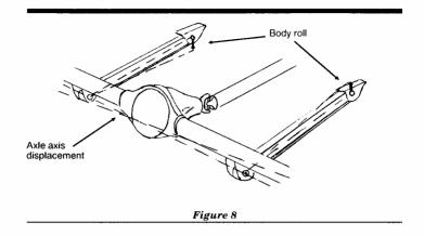
If the frame moves down one inch on one side and up one inch on the other due to a pavement undulation (or gust of wind, etc.), we have the following happen:
