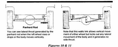
the body and axle, and, thus, reduces the resulting rear tire drift but does not eliminate it. The same effect is caused by upper struts that are angled sharply to act as lateral locator links as on most GM rear drive cars.
