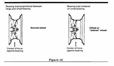
Our recommendation is to use the widest rim your car can take – font and rear – without going to the reversed type, and to keep the same width front and rear, unless you purposely use a rim width difference to balance your drift. A difference between front and rear rim width will require different size tires, front and rear, which complicates tire rotation.
