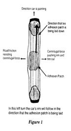
adhesion point is the point at which the lateral force pushing the tire is equal to the friction between the tread and the road surface. If more lateral force is added, then in addition to the drift, you have slide. The more weight you have on the tire, the higher the friction and, therefore, the higher the adhesion point. Extra weight on any given tire will increase both drift and adhesion force.
