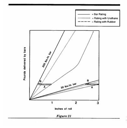
Urethane bushings can be used on the street on most applications. On applications where there is a great amount of suspension travel (such as on the rear suspension of cars, suspensions that are subject to extra load or for off-road use) rubber bushings should be retained at the bar eyes. One can mix rubber & urethane bushings for an intermediate effect.
