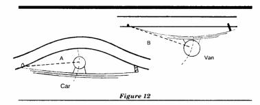
carrying a load. The slope of arc-producing spring A is more horizontal than slope of B on the van; thus, the steering effect is less pronounced. The most direct and most used cure is the addition of anti-sway bars, but this must be carefully done if the car in question has a steep roll axis.
