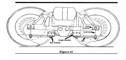
Another example of using a wide suspension width can be seen in the newer 2000-2005 Monoco motorcoaches. The air springs are located just in front and rear of the wheels gaining stability at the full width of the coach thus giving great stability even at mild air pressure, and thus assuring a soft ride. The un-sprung weight is increased by the large framework but the increase stability is worth the slight decrease of ride quality.
