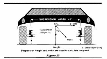
In the foregoing example, the body rolled until the compressing outer spring and the decompressing inner spring were finally able to neutralize the centrifugally displaced mass.
