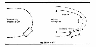
Figure 3 represents the track a car would have to make if it were to execute a continuous-radius 180° curve from a straight line course and then return to a straight line path, such as if a driver tried to follow exactly the wall of an oval track. Actually this would be impossible for the person or the vehicle to do for two reasons:
