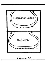
Radial ply tires' greatest virtue, though, is in their behavior under lateral stress during hard cornering
