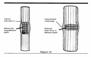
The above illustrates the tire patches of 18 square inches each: One on a four-inch wide tread and the other on an eight-inch wide tread.
