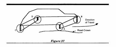
Thus the addition of the front bar reduces body roll, but increases the uneven loading of the tires as the car moves over the side crown of the road. The addition of a front bar only would also crease the loading of the front outer tire due to centrifugal mass shift resulting from the higher roll resistance.
