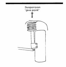
"Strut" suspensions can have very good "suspension width" giving approximate stability to support ratio of 1: 1.4
