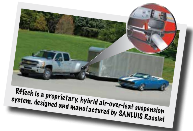
A complete R4Tech kit includes leaf springs, trailing links with J-springs, air springs, load adaptive shocks, air compressor and tank, and all necessary hardware.
