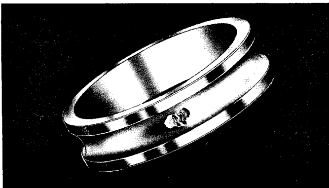
Figure 1. Raceway metal breaking down causing flaking or spalling.
