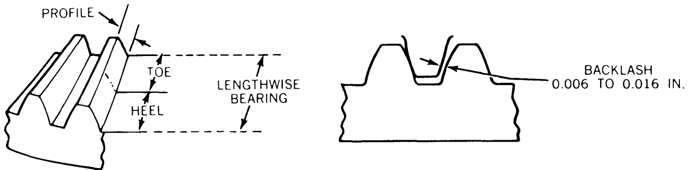
Fig. 26. Ring Gear Tooth Nomenclature
