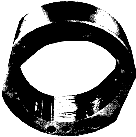
Vane Pump Ring Worn Due to Lack of Lubrication
