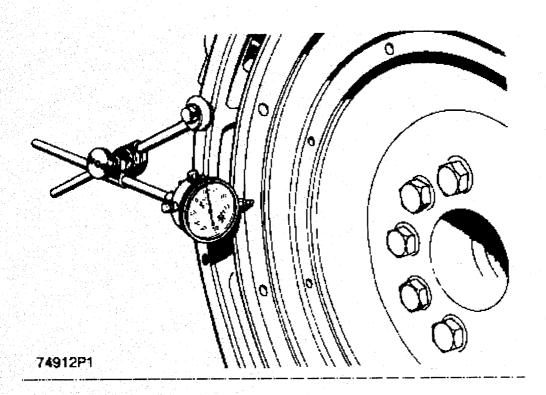
Checking Face Runout Of The Flywheel
