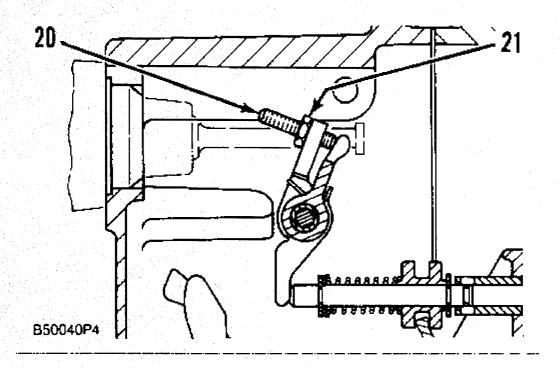
Location Of Linkage Adjustment (20) Adjustment screw. (21) Locknut.
