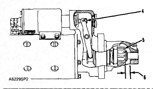
Pinion Clearance Adjustment
