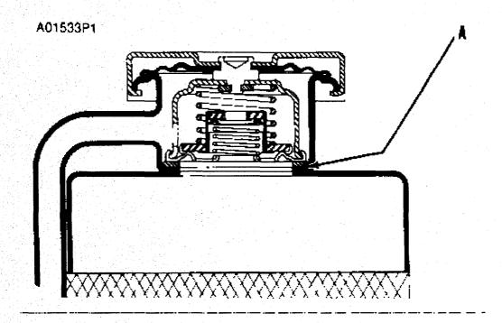
Typical Schematic Of Pressure Cap
