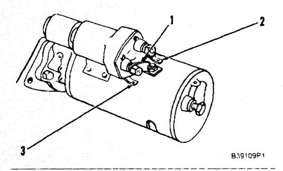
Connection For Checking Pinion Clearance
