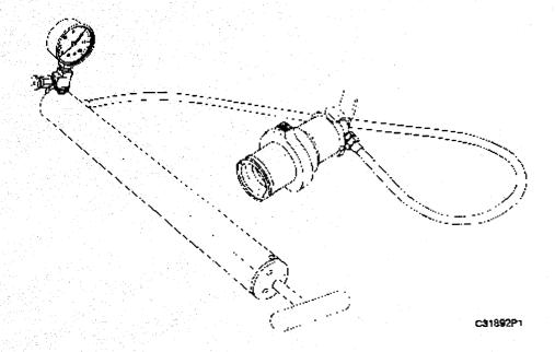
9S8140 Cooling System Pressurizing Pump Group
