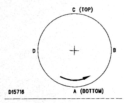
Checking Face Runout Of The Flywheel Housing (A) Bottom. (B) Right side. (C) Top. (D) Left side.
