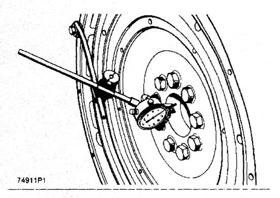
Checking Flywheel Clutch Pilot Bearing Bore
