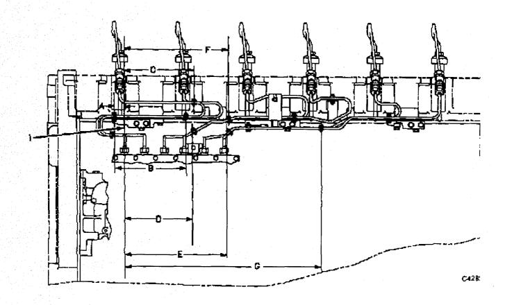
Fuel Injections Lines With Support Bracket
