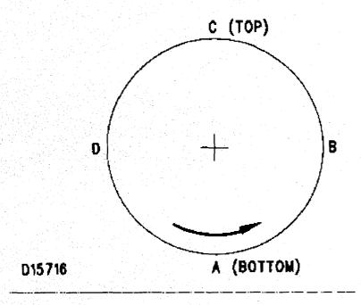
Checking Bore Runout Of The Flywheel Housing
