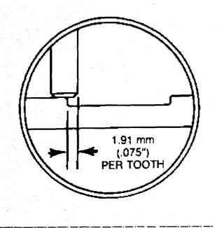
Illustration 2. Incorrect installation, full load position restricted by less than full rack travel.
