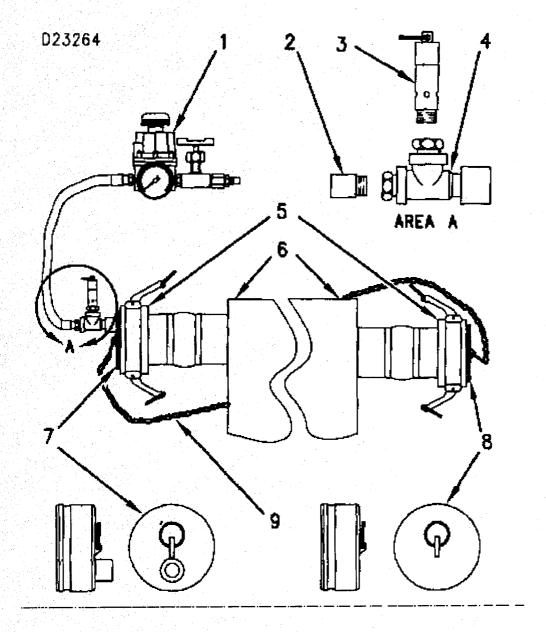
Using FT1984 Air-To-Air Aftercooler Test Group (1) Regulator and valve assembly. (2) Nipple. (3) Relief valve. (4) Tee. (5) Coupler. (6) Aftercooler. (7) Dust Plug. (8) Dust plug. (9) Chain.
