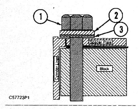
Liner Projection Components (1) Bolt. (2) Washer. (3) Washer.
