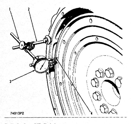
Checking Bore Runout Of The Flywheel
